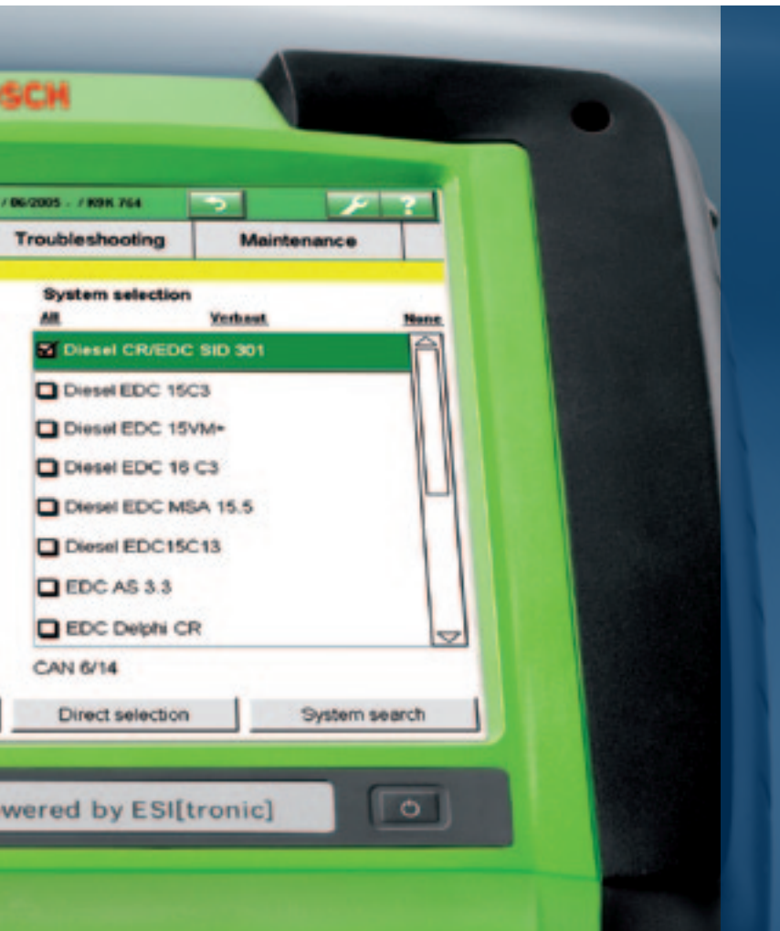
Vehicle information: All higher-order information on the vehicle: Details, systems and diagnostics socket
