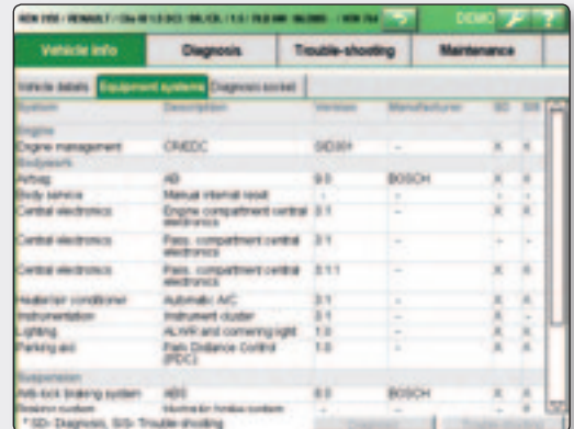
Vehicle information: All higher-order information on the vehicle: Details, systems and diagnostics socket
