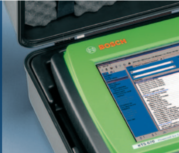
KTS 670: Core element of a professional diagnostic system
